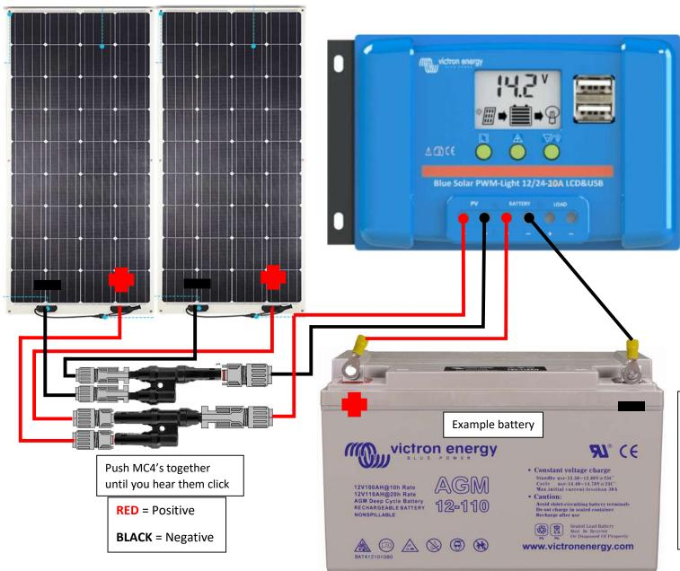
Connect the battery cables first, then the solar.
